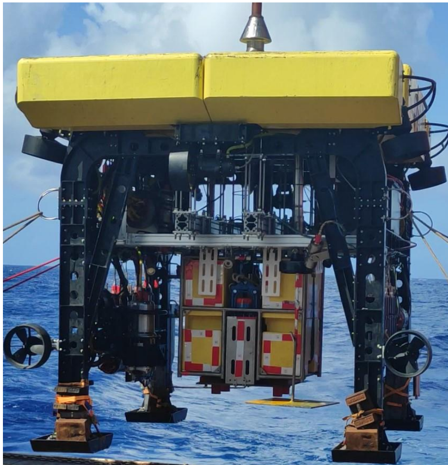
Figure 9-21 ROV-based precision deployment/retrieval system
