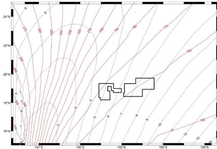
Figure 4-15 S_2 tidal constituent co-amplitude contour lines (in blue, unit: cm) and the co-phase lines (in red, unit: ^\circ )
