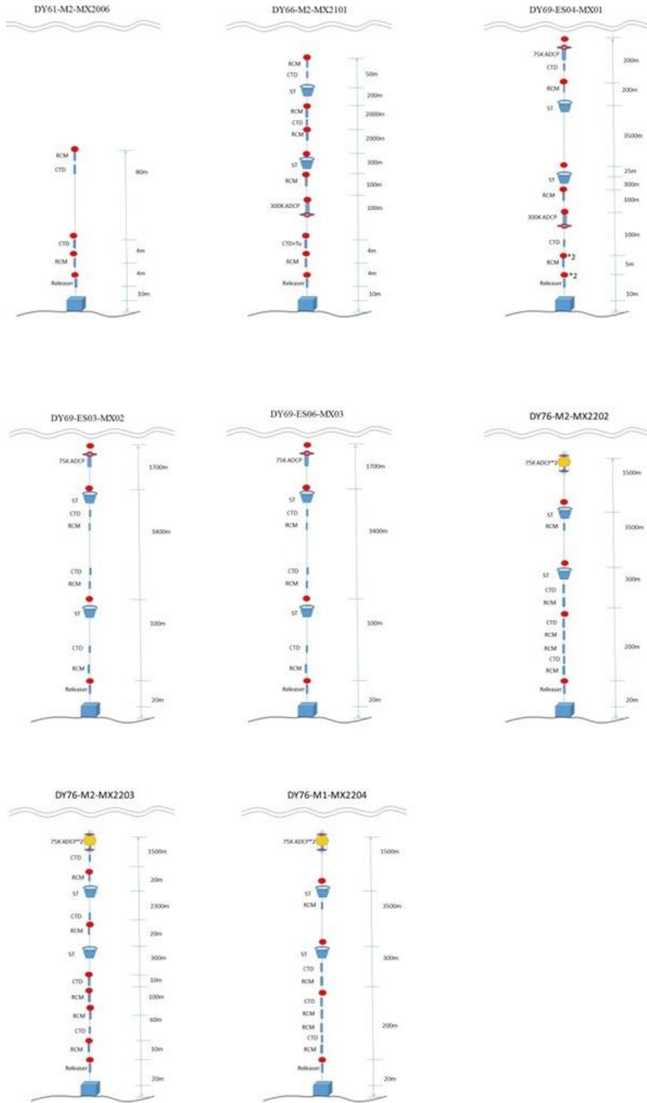
Figure 2-1 Structure of the subsurface buoy
