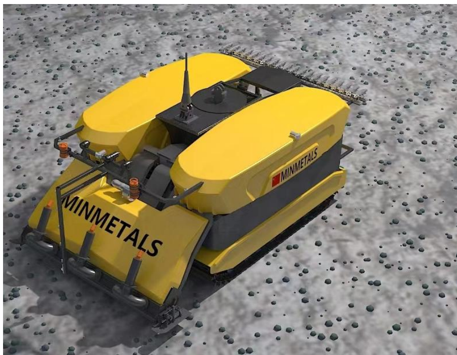
Figure 1 Conceptual model of Minmetals' collector vehicle
