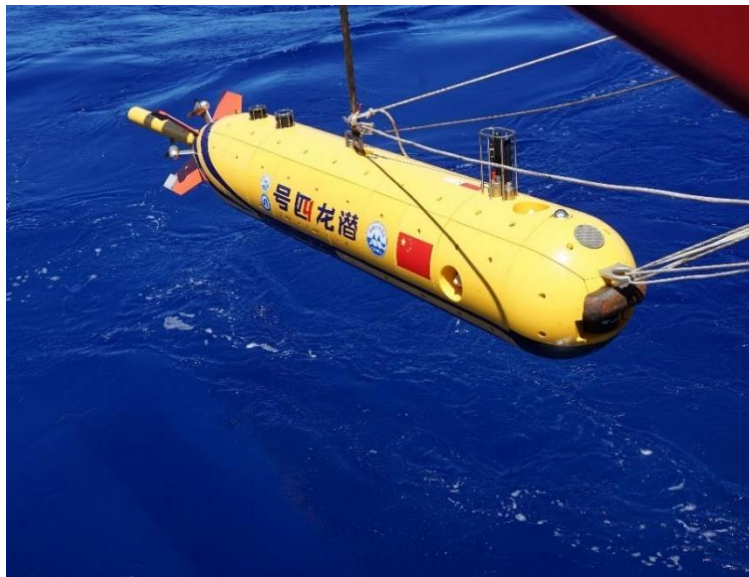
Figure 10.3-10 AUV QIANLONG-IV to be used for near-bottom monitoring
