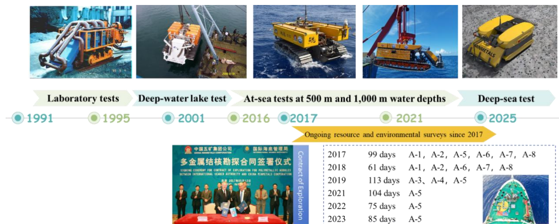
Figure 1.4-1 Development and testing of Minmetals' collector vehicle
