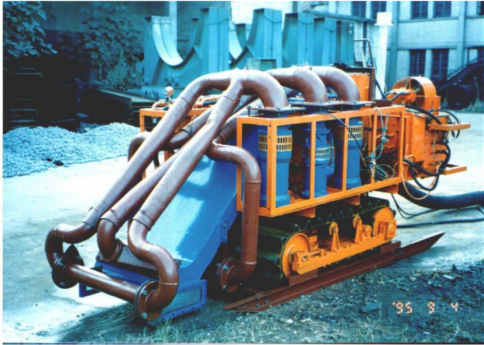
Figure 1.4-2 Prototype of hydraulic collector vehicle
